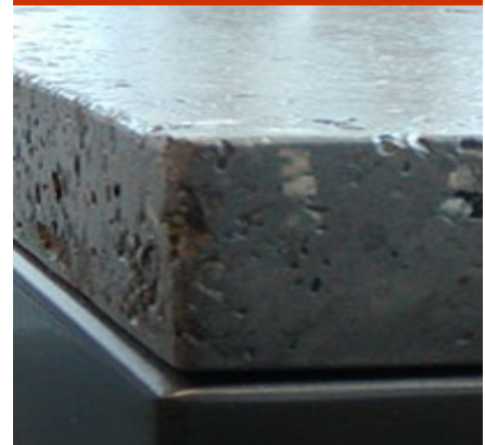
Although slabs are made in standard sizes, each slab is unique. The air holes on the edges are left exposed and unfilled because it gives the product a more natural look.
